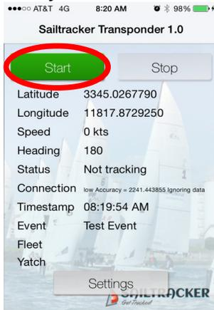
Screen changes to black and tracking is working when Connection reads “GPS OK”
